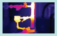
A properly operating steam trap Not all hot spots indicate a problem. This image shows a steam trap that is operating properly. Faulty steam traps waste energy; infrared thermography is an invaluable tool for readily detecting them so they can be repaired.
