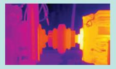
Under-lubricated motor bearing
